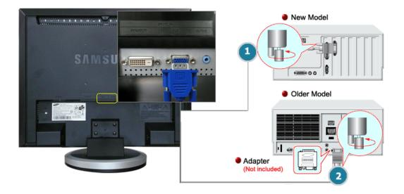
Using the D-sub (Analog) connector on the video card.
